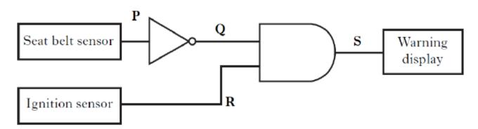
The seat belt sensor produces logic 1 when the seat belt is fastened and logic 0 when the car ignition is off.
