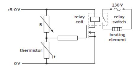
As the temperature of the water increases, the resistance of the thermistor decreases.
