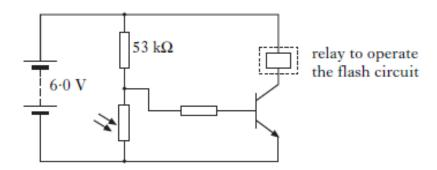
(i) Calculate the voltage across the 53 kΩ resistor when the voltage across the LDR is 0.7 V.
