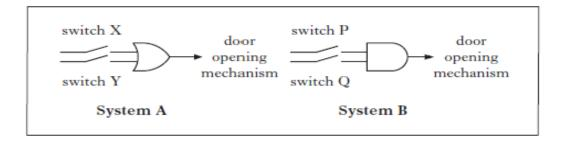
To open the passenger doors on a train, the button marked "Open Doors When Illuminated" must be pressed. To illuminate the button the conductor closes a master switch using a key.
