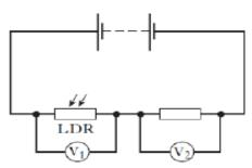
The initial reading on both voltmeters  $V_1$  and  $V_2$  is 2.5 V.
