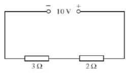
The potential difference across the  $2\Omega$  resistor is
